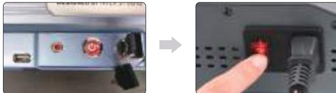
**EN** Turn on the machine power switch first and then turn on the fiber laser control box switch to avoid about 2 seconds ' probabilistic light emission after power on.
